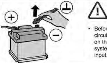
Disconnect the negative terminal on the battery. Make sure the battery cannot unintentionally restart.
