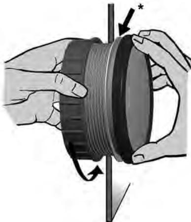
Align the instrument and hand-tighten the fastening nut. Ensure that the nut is not tightened with a torque greater than 400 Ncm.
