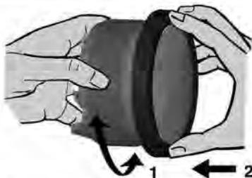
Place the new front ring on the instrument, rotate it until the ring's lip locks into the slots in the housing and press the front ring until it is flush with the instrument glass.
