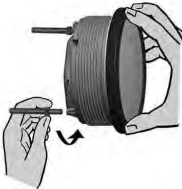
If you would like to omit the fastening nut, you may use the part set A2C59510854 as an alternative. This is recommended if the installation location is subject to vibratory loads. Screw the stud bolts into the provided drill holes in the enclosure. Max. stud bolt torque is 1.5 Nm
