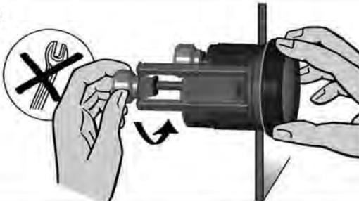
Place the bracket on the stud bolt and hand-tighten the knurled nut.
