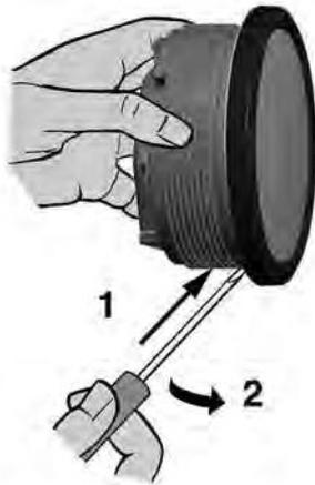
If the instrument is mounted flush (i. e., from the back so that the instrument glass and the panel form one plane), the front ring must be removed. Press the instrument glass with both thumbs, while at the same time pressing the front ring forward from the instrument with both index fingers. Note the use of a tool in the adjacent figure.
