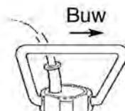
Note the correct direction when inserting the sending unit. The pointed side of the sending unit loop must be directed towards the bow as soon as the sending unit has been inserted.
