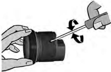
The gauge must be calibrated to the connected immersion tube sensor. Adjust the setting with an insulated screwdriver when the tank is **empty**. Rotate the potentiometer until the gauge reads empty (0 or E). The potentiometer's setting range is between 60 and 90 .
