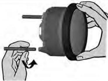
If you would like to omit the fastening nut, you may use the part set A2C59510854 as an alternative. This is recommended if the installation location is subject to vibratory loads.
